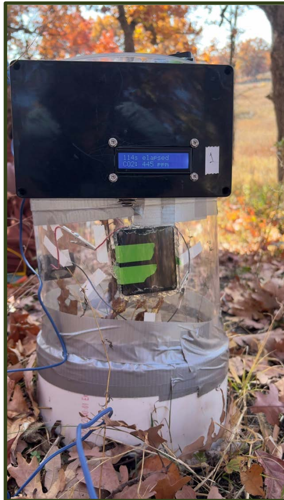
Figure 2. Transparent net carbon dioxide flux chamber including mounted Arduino based automated measurement system
